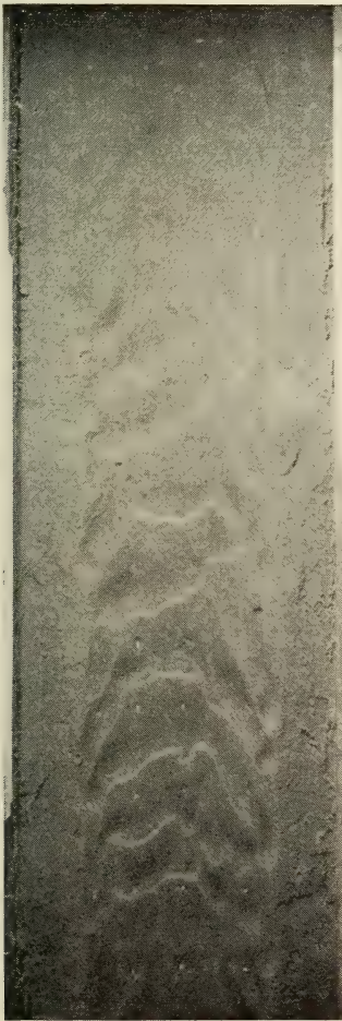
FIG. 17.—Photogrammetric mapping of sand beds in a hydraulic test flume. (The white spots are heads of tacks used as vertical accuracy test points.)
