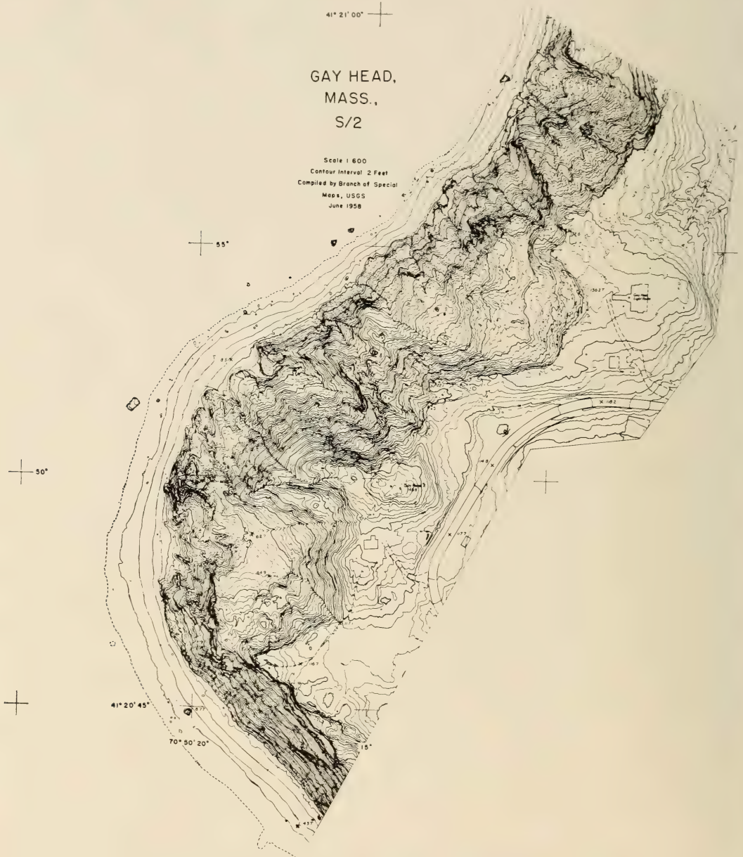
FIG. 16.—Large-scale map for beach erosion study, Gay Head, Mass. Scale 1:600; contour interval 2 feet. Made with Kelsh plotter.
