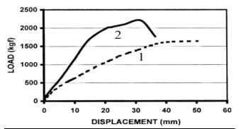
Fig. 2.2. The load-displacement diagram of the "in-bending" loadings of two instances of the mentioned slabs (made according to the system as the ECRLC) "with and without the supplementary bars" in a manner similar to the ASTM E 72 standard
