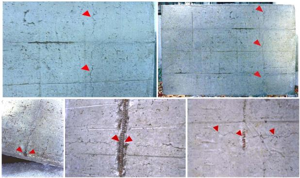
Fig. 2.5. The beneath surface of the tested slab having the supplementary bars after the in-bending loading - The "extended" crack in the expected area (considering the loading manner) is clear.
