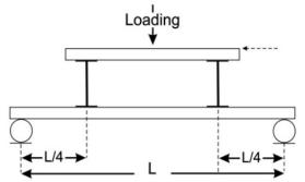
Fig. 2.1. The manner of "in-bending" loadings of the instances of the mentioned slabs (made according to the system as the ECRLC) in a manner similar to the ASTM E 72 standard
