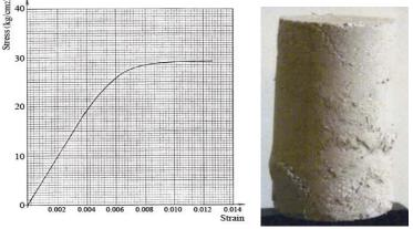
Fig. 1. The stress-strain diagram of in-compressing loading of the pointed lightweight concrete containing the Expanded Polystyrene (EPS) beads as the lightweight aggregates.
