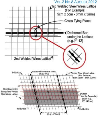
Fig. 4. An Instance of the execution manner of a type of the mentioned ceiling with using the said elements and components (in form of the usual ceilings called as Composite)
