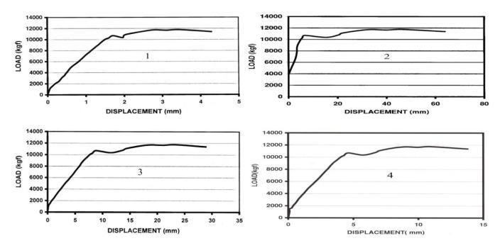
Fig. 3.3. The load-displacement diagrams of the in-compressing loading of an instance of the mentioned slabs (made according to the system as the ECRLC) having the supplementary bars
