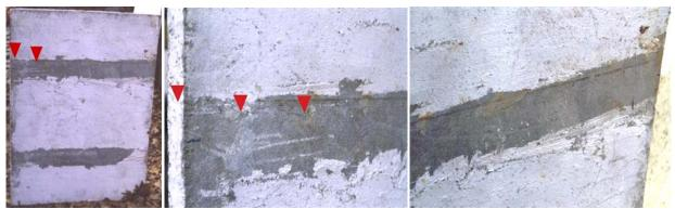
Fig. 2.6. The above surface of the tested slab having the supplementary bars after the in-bending loading - Only a "limited (non-extended)" crack ("having short length and not deep, and in a certain area under the external edge of the employed girder for loading") is obvious.
