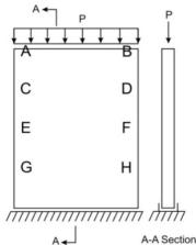
Fig. 3.1. The manner of "in-compressing loading" of the instance of the mentioned slabs (made according to the system as the ECRLC) having the supplementary bars in a manner similar to the ASTM E 72 standard
