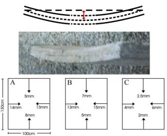
Fig. 2.3. The amounts of the unwanted, asymmetrical primary deflections in the centers of the tested slabs' sides (concerning horizon line) before loading (mm)
