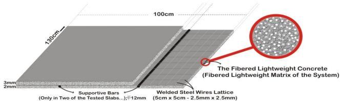
Fig. 2.4. The structure and related dimensions and quantities in the tested slab (made according to the mentioned system as the ECELC) with the supplementary bars [also including the simple recipe (mixture plan) of the used fibered lightweight concrete (as the fibered lightweight matrix) and the said structure in detail for any repetition of the tests]
